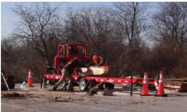
A beneficial reuse contractor cutting slabs from trees to make benches at Floyd Bennett Field.
