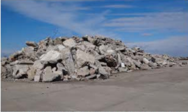
Concrete that has been crushed for recycling at Jacob Riis Park, Queens.
